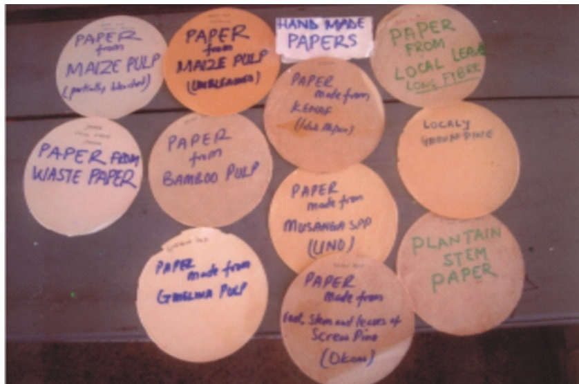
Figure 7: Handmade papers from a locally available paper making raw materials (fibrous and non-fibrous)
